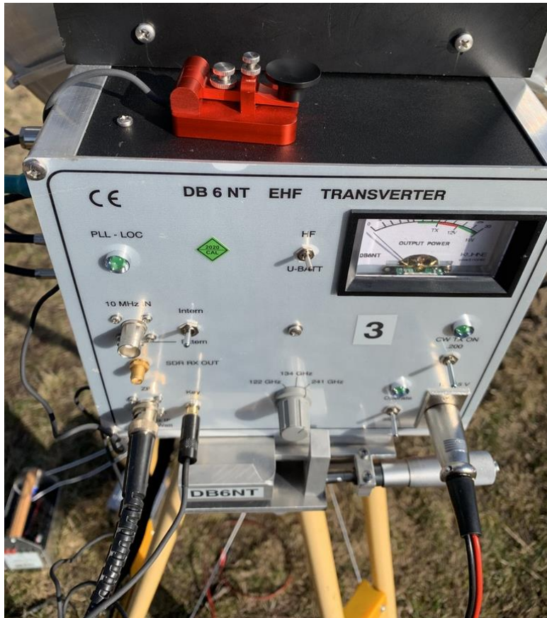
Working condx with the new 241 GHz setup at DK5NJ (the Transverters for 122/136 GHz are also intended to be in this case but this project isn't finished yet)
