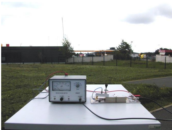
Level measurement with horn antenna
